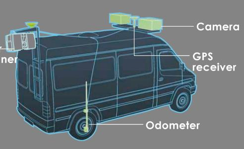
of the environment every three meters as the vehicle moves along. An odometer records the distance the vehicle travels as its coordinates moving through space are tracked and captured simultaneously via a GPS receiver. This data is then collated and stored by an on-board computer, and processed later by the Laser Scanner software.
