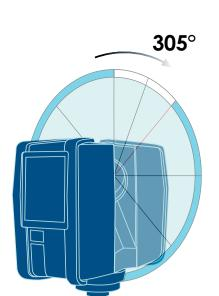
Horizontal angle THE LASER SCANNER revolves 360° horizontally. The horizontal angle is encoded simultaneously with the distance measurement.
