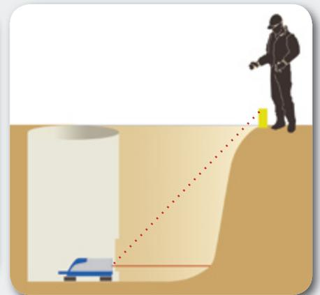
**LINE SET:** The Line Set/Check capability of the pipe laser allows you to raise the beam outside of the trench for fast line setup or checking. Raising the laser beam out of the trench to an above-ground stake saves you time—instead of having to move the excavator off line during setup of the pipe laser, you can just get on with your job. In addition, the Line Set-Check feature is ideal for rechecking the line in pipe jacking puts after each push. Only available on the DG711.
